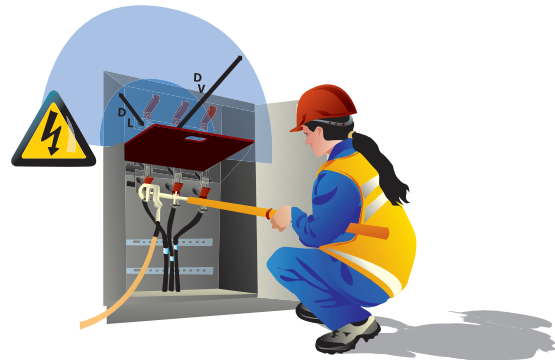
Figure 3. Screen with an insulating board.
