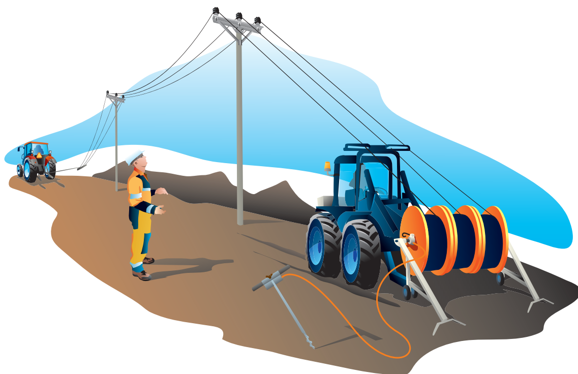
Figure 18. Example of potential equalization to earth when running out a line.
